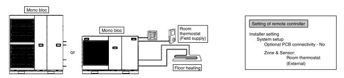
Connect floor heating or radiator directly to Mono bloc.
