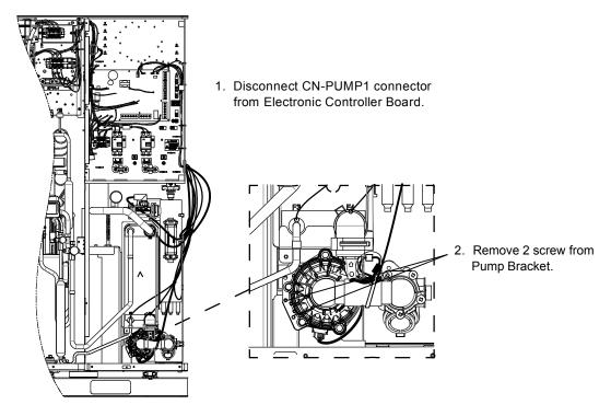
$\bigwedge$  When reinstall the water pipe, use grease or water at the joining.
