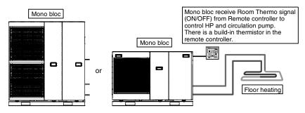
Connect floor heating or radiator directly to the Mono bloc. Install the remote controller in the room where floor heating is installed. This is an application that uses remote controller as Room Thermostat.
