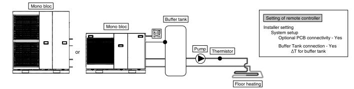
This is an application that connects the buffer tank to the Mono bloc. Buffer tank's temperature is detected by buffer tank thermistor (specified by Panasonic). This system requires optional PCB (CZ-NS4P).
