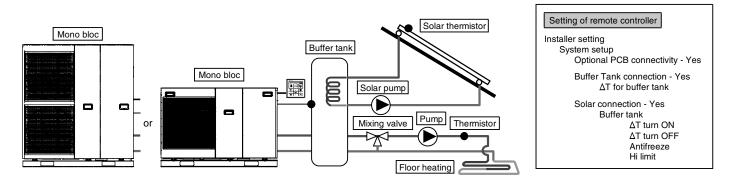
This is an application that connects the buffer tank to the Mono bloc before connecting to the solar water heater to heat up the tank.
