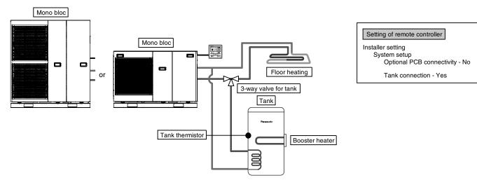
This is an application that connects the DHW tank to the Mono bloc through 3-way valve. DHW tank's temperature is detected by tank thermistor (specified by Panasonic).
