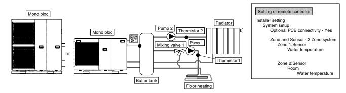
Connect floor heating or radiator to 2 circuits through buffer tank as shown in figure.
