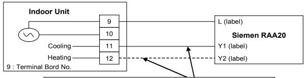
Connect only heating line for heating only model. And connect both heating and cooling line for heat + cool model.
