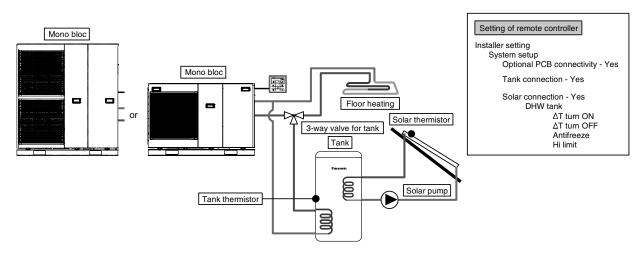
This is an application that connects the DHW tank to the Mono bloc through 3-way valve before connect the solar water heater to heat up the tank. DHW tank's temperature is detected by tank thermistor (specified by Panasonic). Solar panel's temperature is detected by solar thermistor (specified by Panasonic).
